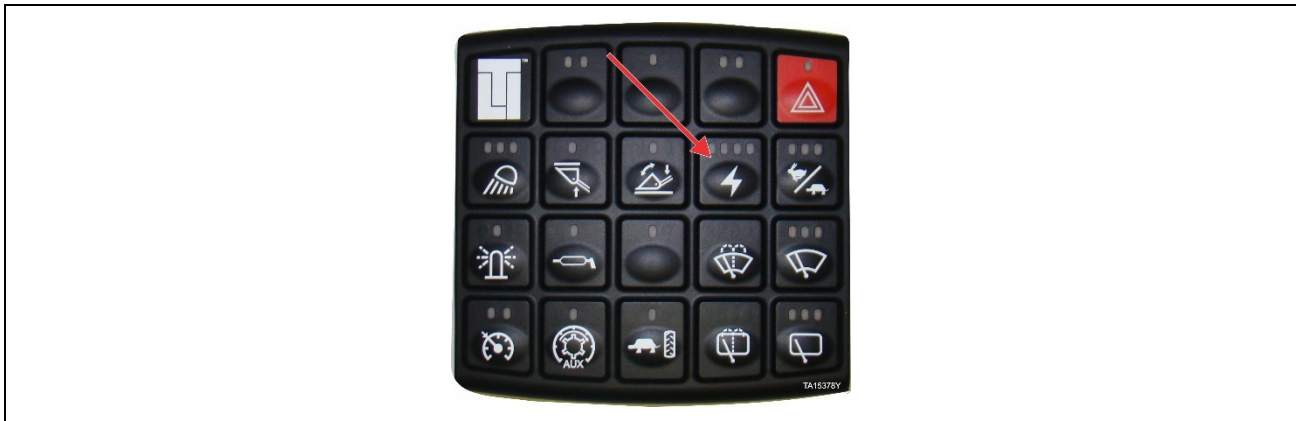
Figure 16. Drive Enable Switch
